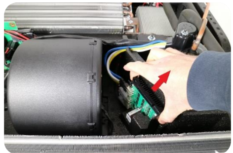
3) Slide out the main PCB
